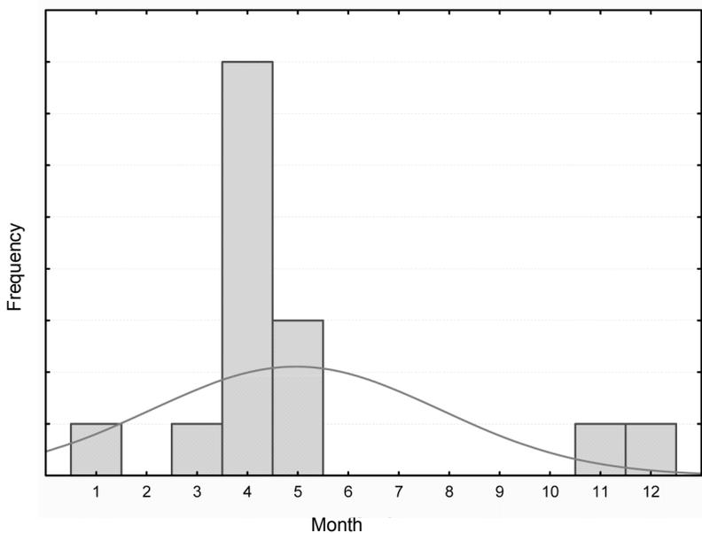
Fig. 3. Frequency of recorded absolute monthly maximum water level of the river Danube in Silistra hydrometric station for the period 1994–2008
